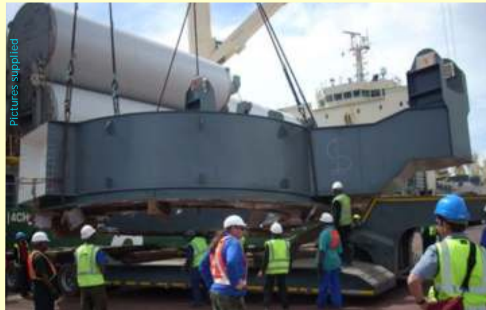
Cargo operations at Durban harbour where a ship alongside is discharging a heavy lift steel structure onto a flat bed trailer on the quayside. Stevedores are conducting the operation and a cargo surveyor, wearing a blue hardhat, is monitoring the operation for insurance purposes
